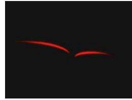
(b) Camera image for the light stripe triangulation.
