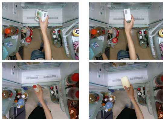
Figure 3. The images captured by the camera. The groceries are occluded by user's hand and their visible portion is inconsistent.
